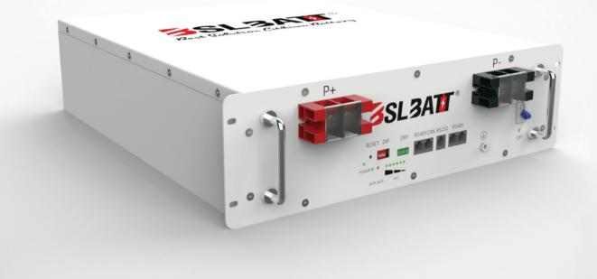
B-LFP48-100E 3U 51.2V 5.12kWh with 100A internal BMS. Composed of (16) UL listed prismatic 3.2V LiFePO4 cells in series which have been tested at 6000 deep discharge cycles to 80% DoD - fully charge and discharge this battery daily for over 10 years without issue. You'll get 10 years of warranty service and technical support with BSL inverters and batteries!
